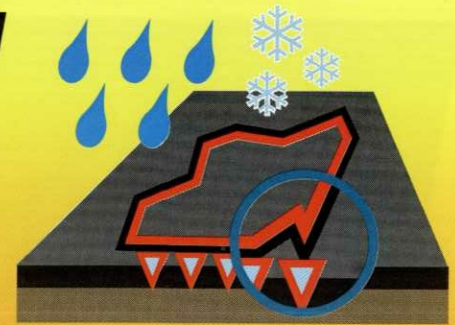
Problem: Frost danger caused by cracks and holes
